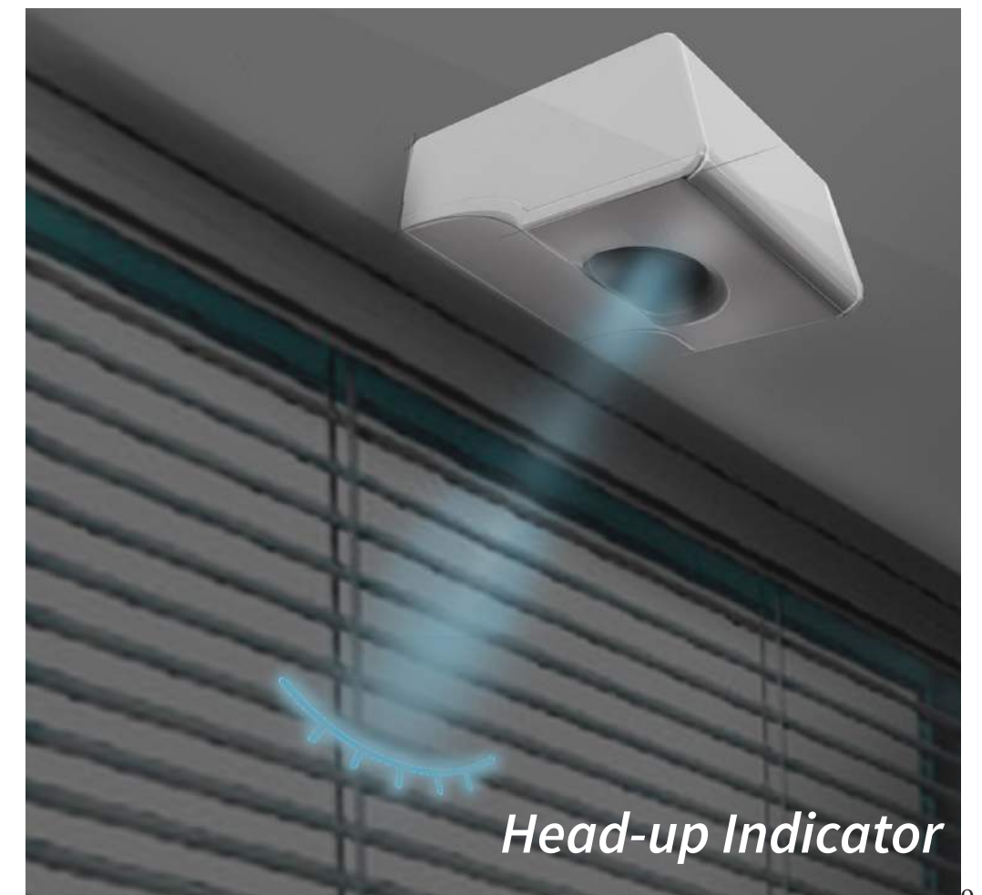
Figure 2.3 The sleep status indicating device of SLEEG
