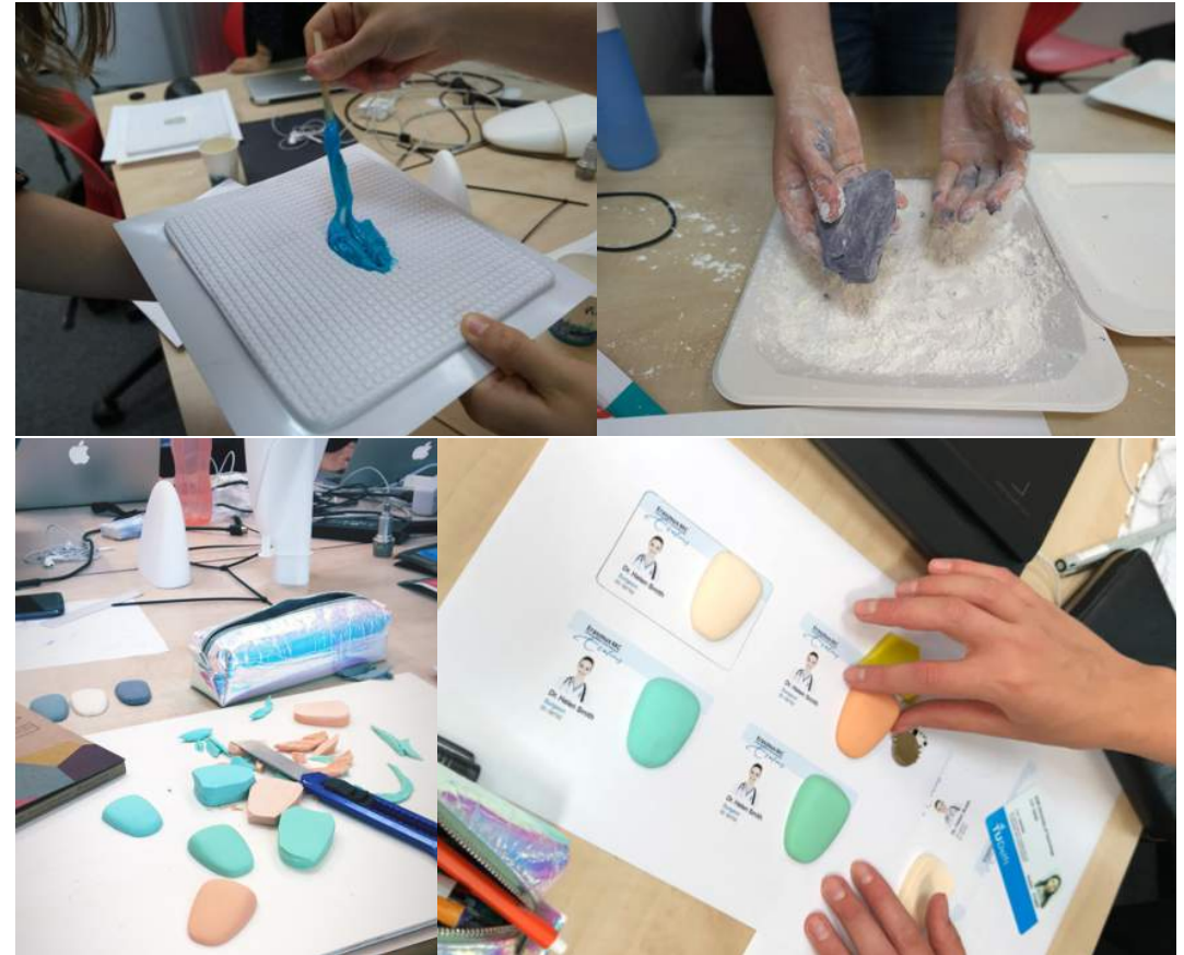
Figure 4.1.3: Molding and cutting silicon model
