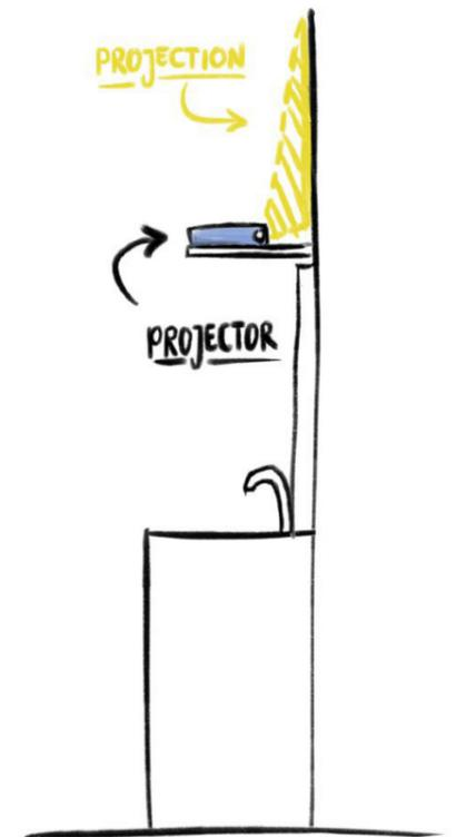
Figure 62: Placement beamer close to wall.
